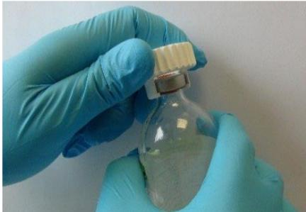
Select the adapter for the corresponding bottle. Insert the bottle into the universal adapter
