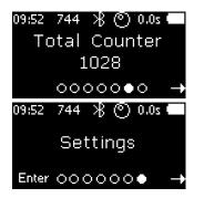
The sixth page shows the Total Counter, which counts the total number of injections. This counter cannot be reset as it is a key indicator of the age of the device.
