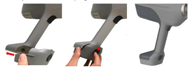
A fastening button will hold the battery in position. The battery can be removed from the base by pushing down the button at the front of the battery and by pulling out the battery.
