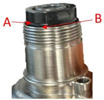
**Attention:** The groove must remain visible, i.e. it must not lie below the edge or become invisible. If the groove lies below the edge, the cylinder is screwed in too far and will harm the functionality of the device.
