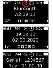
On the third page, Bluetooth can be controlled. Push the left display button to disable or enable the Bluetooth antenna. If using the HSW Connect App, enabled Bluetooth is required.
