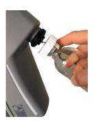
d. Pre-puncture the stopper of the vaccine bottle centrally with a sterile needle to avoid rubber particles being drawn into the spike of the vaccination device and eliminate the overpressure inside the bottle. Place the injector on a solid surface (as shown on the first picture) and push the bottle onto the spike using the pre-punctured hole.
