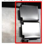
Pull the drawer out of the device until two metal flaps are visible and can be moved.
