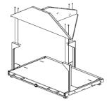
Take the cover as shown on the left and place it on the pillars that have already been mounted to the main casing. Take care to place it onto all three pillars to prevent it from falling prior to fixing in place with screws.
