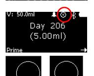
This sensor allows for continuous control of the correct holding position of the device (see picture on the left). Once the injection is done and before allowing liquid to be drawn into the device the position sensor will check if it is held upright in order to avoid drawing in air.
