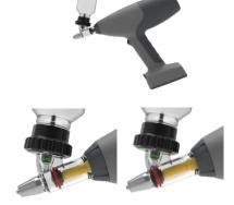
If you want to start to prime the device, first press the trigger button. The device will move the piston forward to the end position (This is necessary to make a reference drive for the motor). When pressing the trigger button again, the piston will move to 20% of the volume for easier priming of the cylinder. Press again and the device will start to prime the device. Check if all air bubbles were removed from the cylinder.
