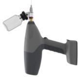
If you hold the device when the needle pointing upwards, the plunger will move only in small steps by pressing the trigger button. When all air is out hold the device in a normal position and press the mode button (P) or finish and you will come back to the vaccination mode.
