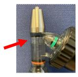
To remove air from the cylinder when there is only a little air in the cylinder (see picture), press the mode button (P) or press the left button to enter the priming mode.
