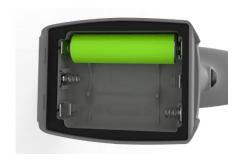
Insert the batteries in the right direction (pay attention to + and -). Before inserting the batteries, check them for mechanical damage. If any damage is obvious dispose of them properly. Make sure to use the correct battery model. Please use 18650 Li-lon PCB protected rechargeable 3,6/3,7V Batteries with a min. capacity of 2600mAh and min. continuous discharge current of 5,2A to ensure full functionality according to the product's specifications.
