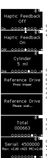
On the fifth page, the haptic feedback can be controlled. Push the left display button to disable (Off) or enable (On) the haptic feedback which will confirm the injection.
