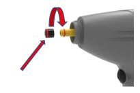
Take the other piston and mount it clockwise onto the thread hand tight.
