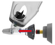
Hold the piston tip and turn it counterclockwise to release it.
