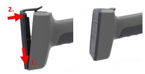
Close the battery slot with the cover properly.
