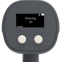
To clean the fluid path (Spike, inlet valve, cylinder, plunger and outlet valve), mount a bottle of Isopropanol or soap solution to the device and set the volume to the highest volume and do 10-20 rinsing cycles to remove all residues by pressing the trigger.
