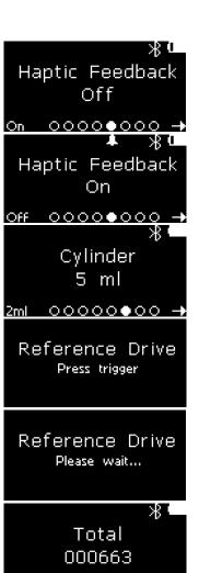
On the fifth page, the haptic feedback can be controlled. Push the left display button to disable (Off) or enable (On) the haptic feedback which will confirm the injection.
