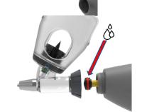
Lubricate the O-ring and then mount the new cylinder.
