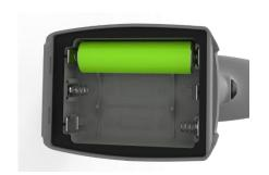
Insert the batteries in the right direction (pay attention to + and -). Before inserting the batteries, check them for mechanical damage. If any damage is obvious dispose of them properly. Make sure to use the correct battery model. Please use 18650 Li-lon PCB protected rechargeable 3,6/3,7V Batteries with a min. capacity of 2600mAh and min. continuous discharge current of 5,2A to ensure full functionality according to the product's specifications.
