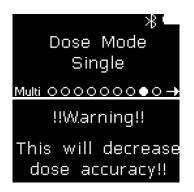
For activating the Multi Dose Mode press the left button for two second. After that a Warning screen will appear, see below.
