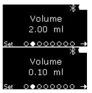
On the second page, the volume can be adjusted. The currently set volume is shown in the center.
