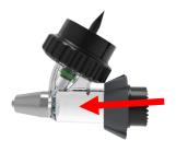
Remove plastic barrel from the handle by turning the nut. Lubricate piston and inside the barrel with 100% pure oil, cold squeezed or equivalent vegetable oil.
